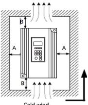
Installation clearance requirements on the MD380 series AC drives of different power classes
